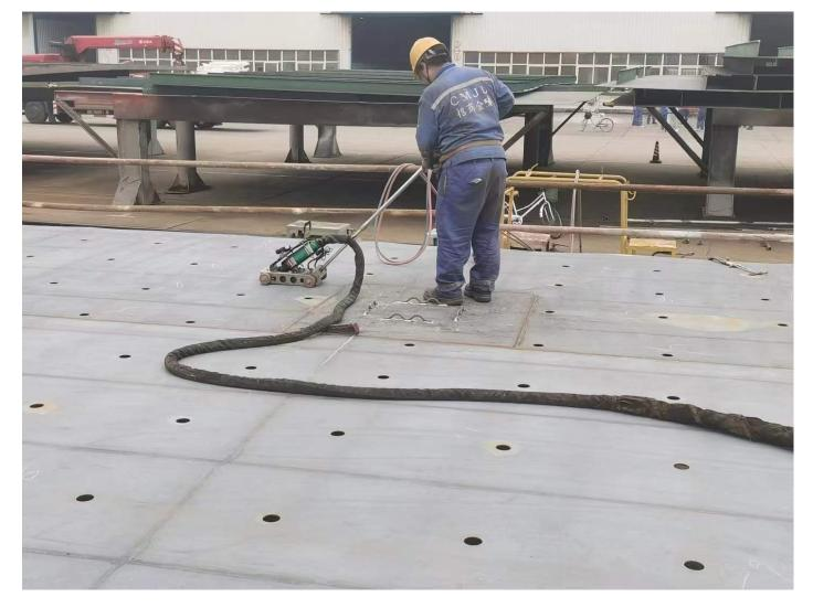
FAQs About Induction Heating Systems for Structural Straightening
