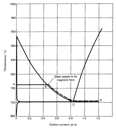
Fig. 2.4 Curie temperature for carbon steels. Source: Ref 2
