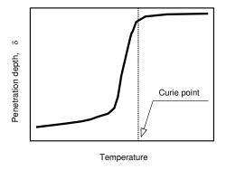
Fig. 2.8 Variation of current penetration depth through Curie. Source: Ref 6
