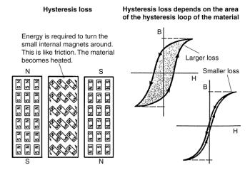
**Fig. 2.3** Effect of hysteresis on heating rate. N, north; S, south; B, flux density in a ferromagnetic material; H, corresponding magnetic intensity. Source: Ref 4
