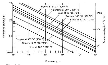
Fig. 2.5 Reference depth for various materials. Source: Ref 2
