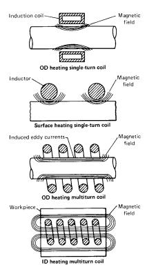
Fig. 2.1 Induction coil with electromagnetic field. OD, outside diameter; ID, inside diameter. Source: Ref 1
