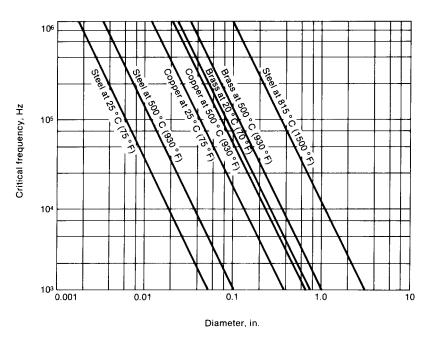
Fig. 2.6 Critical frequency for efficient heating of several materials. Source:
