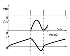
Figure 5-16: Wave Forms At a Non-zero Voltage Turn-On
