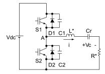
Figure 5-5: Equivalent of the Main Power Circuit
