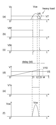
Figure 5-20: Waveform of Each Part In the Control System
