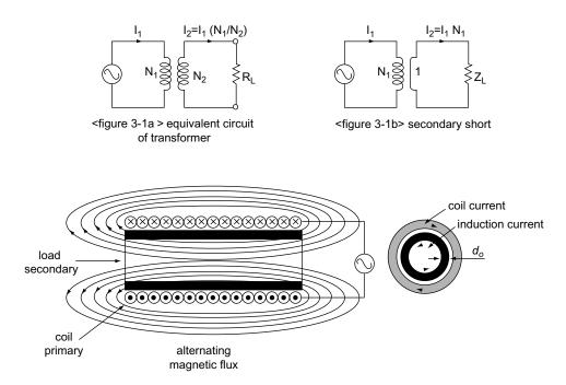
Figure 3-1: Basics of Induction Heating
