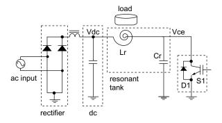
Figure 5-10: Main Power Circuit
