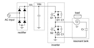
Figure 5-3: Main Power Circuit
