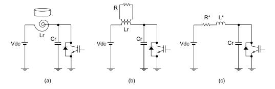
Figure 5-11: The Equivalent of a Resonant Circuit
