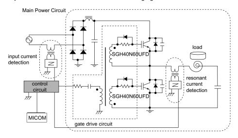
Figure 5-2: Power System Using Half-bridge Series Resonant Converter
