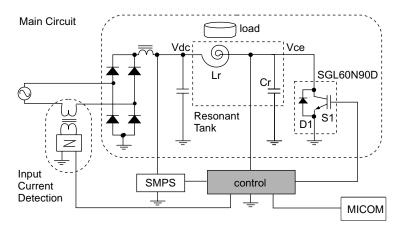
Figure 5-9: Power System Using a Quasi-resonant Converter
