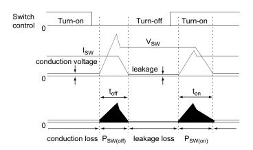
Figure 4-1: Wave Form of a Switching Device
