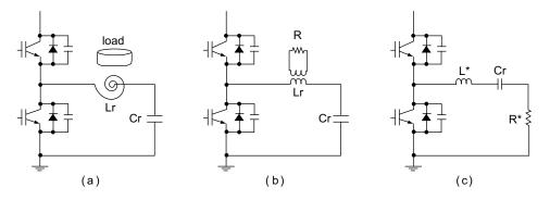
Figure 5-4: Equivalents of the Resonant Circuit
