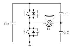
Figure 5-8: Common Type of Main Power Circuit
