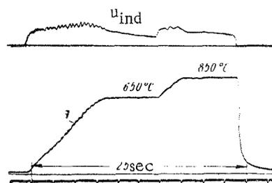
Fig. 8. Induction heating with two isothermal plateaus.
