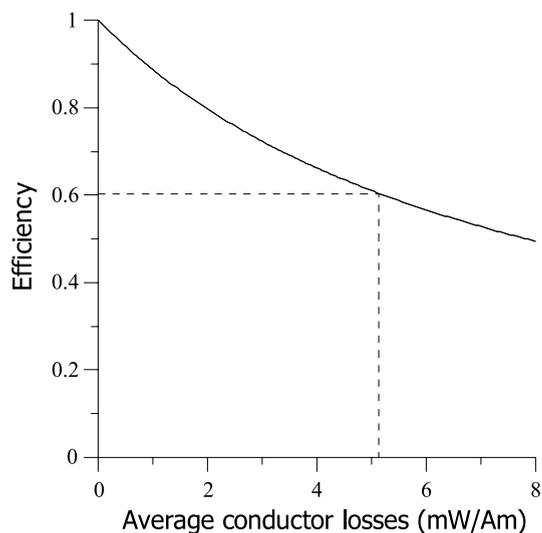
Fig. 2. Calculated efficiency of a 5 kW induction heater as a function of average AC losses in the HTS coil operating at 77 K. A cooling penalty factor of 20 has been assumed and the thermal losses have been neglected. The dashed line corresponds to what can be expected from DC HTS tapes available today.
