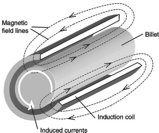
Fig. 1. Principles of induction heating of a massive cylinder (a billet).
